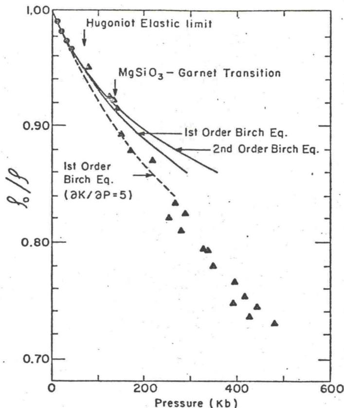
Fig. 7. Comparison of ultrasonic equation of state for bronzite calculated from Birch's equations with static-compression data of *Bridgman* [1948] (circles) and shock-wave data of *Ahrens and Gaffney* [1971] (triangles and dashed lines).
